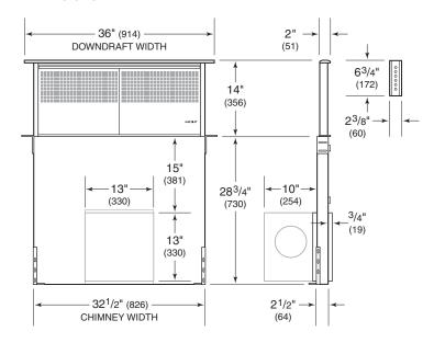
NOTE: Shaded line represents internal blower box with 6" (152) round discharge.
