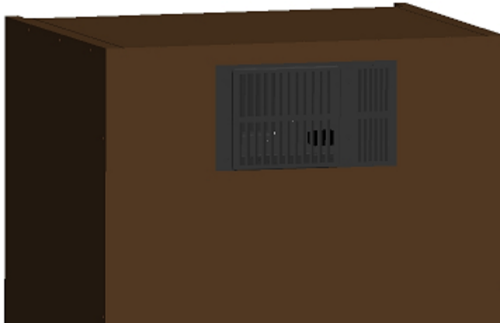
Fig. 2.8 COOLING UNIT MOUNTED (REAR EXHAUST)
