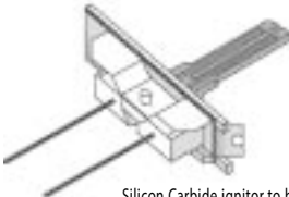
Silicon Carbide ignitor to be replaced.
