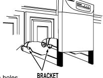
**NOTE:** Hole drill size will depend on size of hardware being used for installation.
