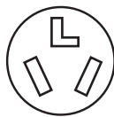
3-wire receptacle (10-30R)
