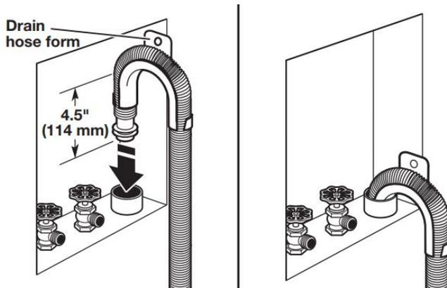
Place hose into standpipe (shown in picture) or over side of laundry tub.
