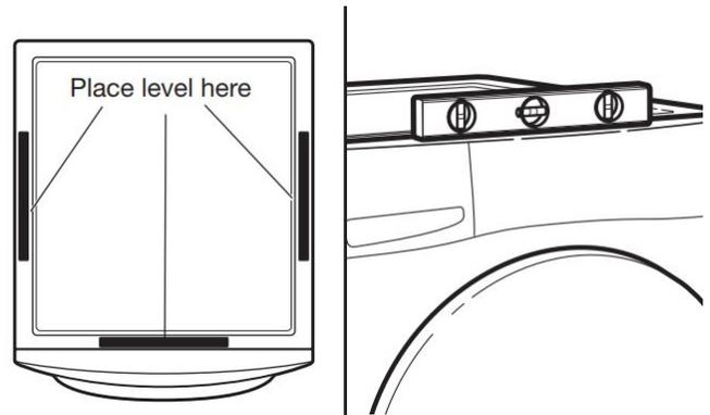
Remove cardboard from beneath washer. Place a level on top edges of washer, checking each side and front. If not level, tip washer and adjust feet up or down as shown in steps 15 and 16, repeating as necessary.
