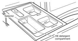
Do not overfill; adding too much detergent may cause detergent to be dispensed into the washer too early.
