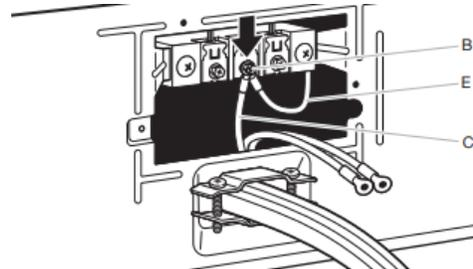
Connect neutral bond wire (E) and neutral wire (white or center wire) (C) of power supply cord or cable under center terminal block screw (B). Tighten screw.
