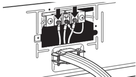
Place remaining wires under outer terminal block screws. Tighten screws.
