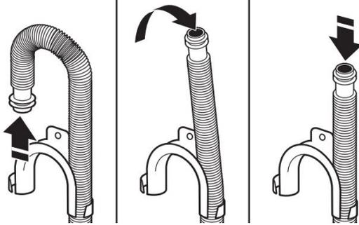
For floor drain installations, you will need to remove the drain hose form from the end of the drain hose. You may need additional parts with separate directions; refer to the Quick Start Guide.
