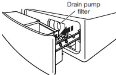
With your finger, push down on tab on right side of drawer, and up on tab on left side of drawer.
