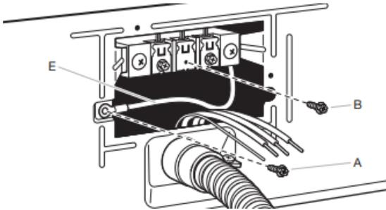
Remove center terminal block screw (B). Remove neutral bond wire (E) from green external bond conductor screw (A).
