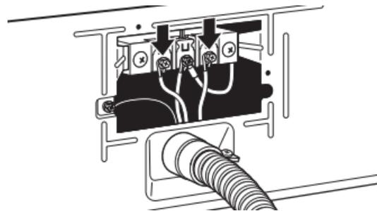
Place hooked ends of remaining direct wire cable wires under outer terminal block screws (hooks facing right). Squeeze hooked ends together and tighten screws. Insert tab of terminal block cover into slot of dryer rear panel. Secure cover with hold-down screw. Now, go to "Venting Requirements."
