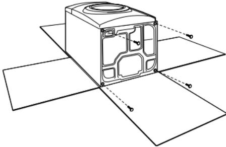
To avoid damaging floor, use a large flat piece of cardboard from dryer carton; place under entire back edge of dryer. Firmly grasp dryer body (not console panel) and gently lay dryer down on cardboard.
