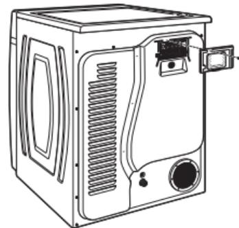
Remove hold-down screw and terminal block cover.
