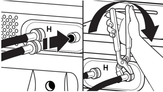
**IMPORTANT:** To reduce risk of hose failure, replace the hoses every 5 years. Record hose installation or replacement dates for future reference.
