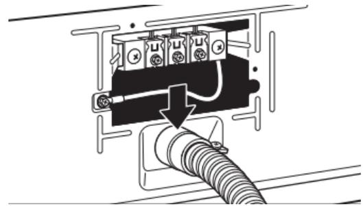
Put direct wire cable through the strain relief. The strain relief should have a tight fit with the dryer cabinet and be in a horizontal position. Tighten strain relief screw against the direct wire cable.
