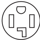
4-wire receptacle (14-30R)
