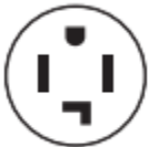
4-wire receptacle (14-30R)
