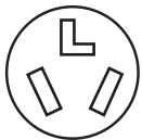
3-wire receptacle (10-30R)
