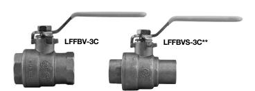
**NOTE:** Apply heat with the flame directed **AWAY** from the center of the valve body. Excessive heat can harm the seats. After soldering, the packing nut may have to be tightened.
