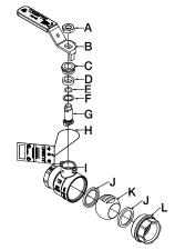
A. Handle NutB. Handle AssemblyZinc plated carbon steel with
