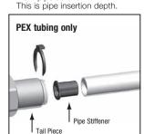
3. If using PEX tubing, insert pipe stiffener (provided) into end of pipe.
