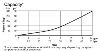
\*Flow curve with integral inlet filters and check valves
