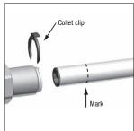
4. Push tubing into tailpiece up to mark. 5. Insert collet clip.
