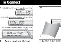
Mark pipe as shown. This is pipe insertion depth.
