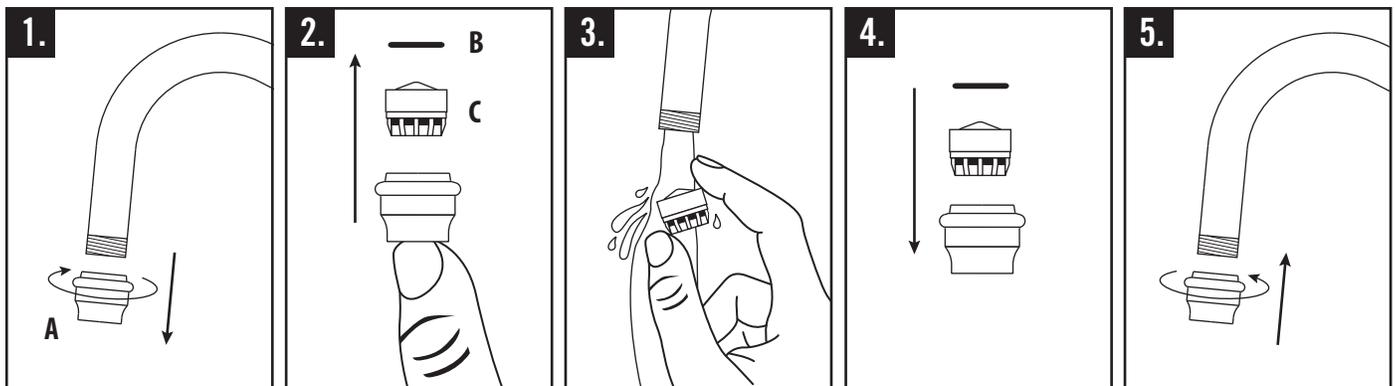
Depending on quality of your household water, the aerator and debris screen may become clogged. We recommend cleaning one week after installation, then a minimum of once of year thereafter. To remove the debris, follow the steps below.
