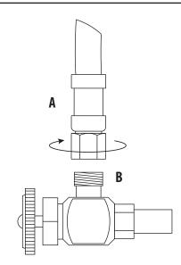
1. Before connecting supply hoses, flush supply stops to clear any debris. Place a bucket underneath stops and run water for 5 to 10 seconds. Turn water off. 2. Carefully position hot and cold supplies so they will not interfere with other hoses. 3. Connect supply hoses (A) to supply stops
