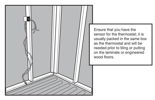
Lay out the cold lead and run to the junction box. DO NOT run the cold lead on top of the mat, run along the edge of the mat. Use a marker to trace the cold leads and mark the splice locations on the subfloor. The cold lead and splice are slightly thicker than the mat, some removal of sub-floor material may be required where the splice will set or where the cold leads will run to eliminate any possible interference with the tile.
