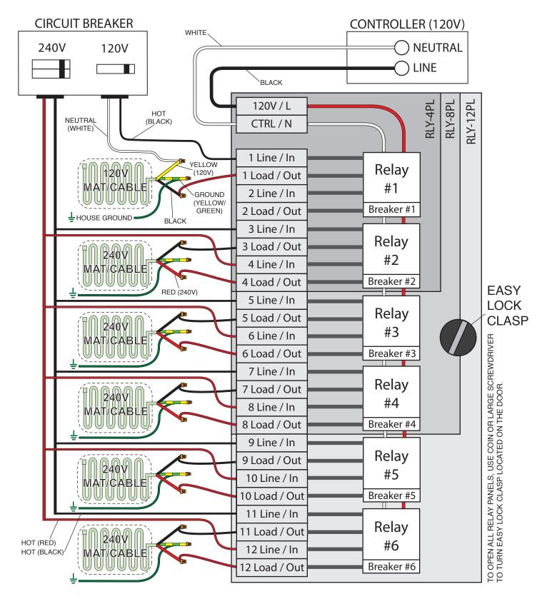
MAXIMUM AMP LOAD PER RELAY IS 30 AMPS
