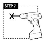
STEP 7: Drill A, B, C, and D holes with an appropriately sized bit. Use a hammer to knock plastic drywall anchor (f) into wall completely.
