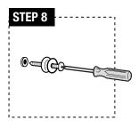
STEP 8: Insert long screw (h) through mounting bracket (g), then screw into plastic drywall anchor (f).
