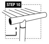
STEP 10: As shown in the picture, install the set screws (c) into the hole of all the tubes (a,b and k) using the allen wrench; fix the tube (a,b and k) onto the mounting bracket (g).
