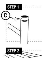
**STEP 1:** Remove and set aside the set screws (c) from the top of the main assembly.
