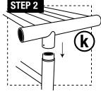
**STEP 2:** Slide the mounting shelf's collared feet (k) over the top of the main assembly so that the mounting shelf is perpendicular to the main assembly.
