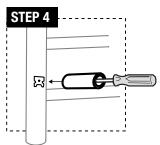
**STEP 4:** Insert the short mounting screw (d) through the tube in the center of the mounting tube (a).
