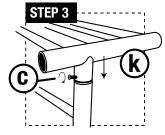
**STEP 3:** Secure the mounting shelf (k) fto the main assembly by using the set screws (c) from Step 1.
