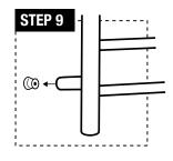
STEP 9: Install the tube (a and b) onto the bracket (g).
