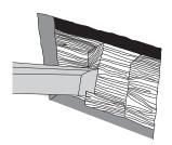
3. The sill plate or bottom plate of the wall may need to be notched with a wood chisel directly below the location of the thermostat to allow placement of the conduit for the coldlead and sensor (if required). There should be a conduit for the cold lead and a separate conduit for the sensor if the local code requires low voltage wires be protected by conduit.
