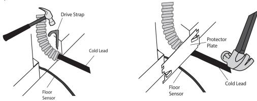
7. Place the smurf/ENT tube over the sensor wire to protect it from the high voltage wires.
