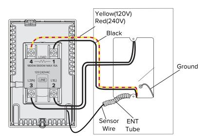
Place the thermostat into the single gang box and line up all of the holes. Use the included screws to attach the power base to the box. Center and level the thermostat and then tighten the screws to hold the unit in place. Install thermostat's faceplate onto the power base.
