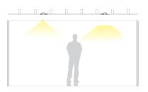
Linear channel can be field cut Accommodates up to four runs of InvisiLED® indoor tape Dense foam insert to be removed in installation after spackling Allows option to use different color InvisiLED® in one channel and switch them separately
