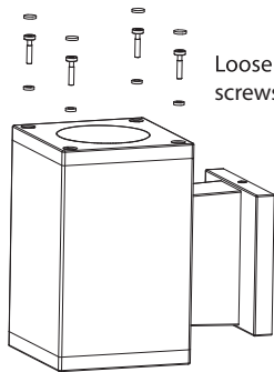
FIG.5 Loosen the fixture screws and gaskets
