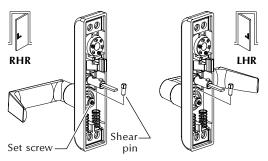
**3.** Install cam with R facing out for RHR or L facing out for LHR.
