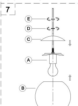
7. Attach glass globe (B) to fixture. Place glass cover (C) to fixture using knurled nut (D) and slip finial (E) to secure tightly.
