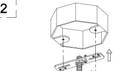
2. Attach assembled parts from Step 1 onto outlet box using the mounting screws supplied with the outlet box (not included).
