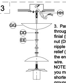
3. Pass the wires through the slip finial (EE)/ knurled nut (DD)/ canopy (GG)/ nipple and strain relief (HH). Tie a knot at the end of the fixture wire.
