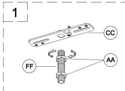
1. Screw threaded nipple (FF) into mounting strap (CC) several turns. Use one hex nut (AA) to secure parts tightly. Screw one hex nut (AA) onto threaded nipple (FF).
