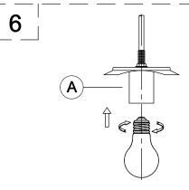
6. Screw bulb (not included) into fixture socket (A).
