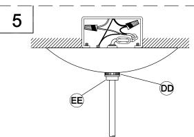
5. Tuck the wires into the outlet box and slip the canopy over the nipple. Thread the finial (EE) and knurled nut (DD) on the nipple to secure the canopy tightly to the ceiling.
