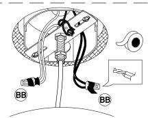
4. Strip 3/8" of insulation from the electrical wire ends. Using wire nuts (BB), connect white fixture wire to the white supply wire from the outlet box; connect the black fixture wire to the black supply wire.
