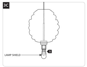
**5** Push the lamp shield onto the spring clip.
