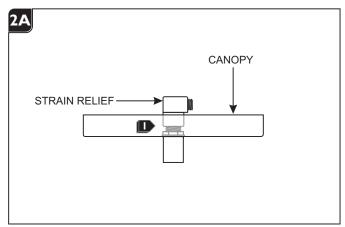
From back of the canopy tighten the strain relief to the cord grip.
