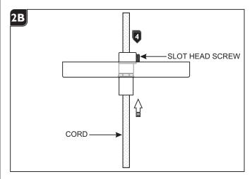
**NOTE:** Refer to the instructions provided with the pendant fixture to install the fixture shade (if needed) before proceeding with these steps.
