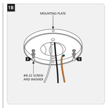
3 Secure the mounting plate to the electrical box with the two washers and #8-32 screws provided.
