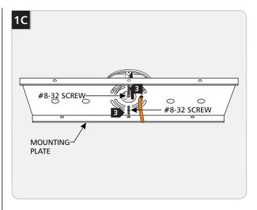
3 Secure the mounting plate to the electrical box with the two #8-32 screws provided.
