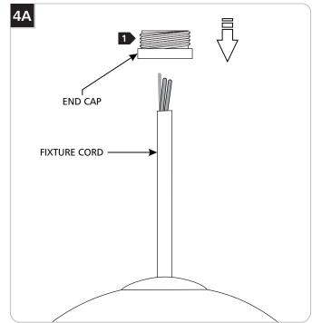
Slide the end cap over the fixture cord making sure the threading faces upward.
