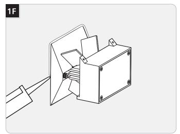
**9** For wet locations, caulk around the base with waterproof construction sealant.
