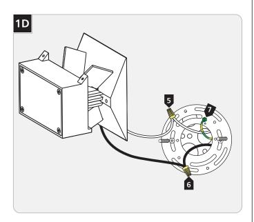
**5** Connect the white fixture wire to the neutral power line wire with a wire nut.
