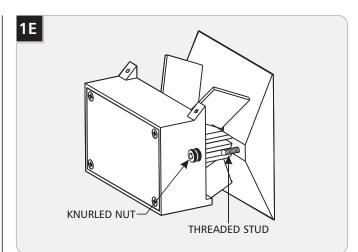
8 Neatly tuck all wires and wire nut connections into the electrical box, mount the fixture onto the threaded studs, and secure it in place by screwing the knurled nuts onto the studs.
