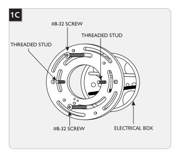
Align the two mounting studs horizontally and mount the mounting plate to the electrical box with the two #8-32 screws provided.
