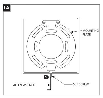
■ With the Allen wrench provided, back out (do not fully remove) the set screw at the base of the fixture and remove the mounting plate.
