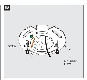
2 Attach the mounting plate to the electrical box using the two #8-32 screws provided.
