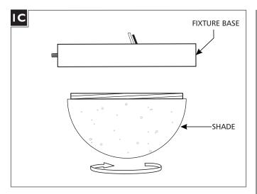
**3** Screw the shade securely into the fixture base.
