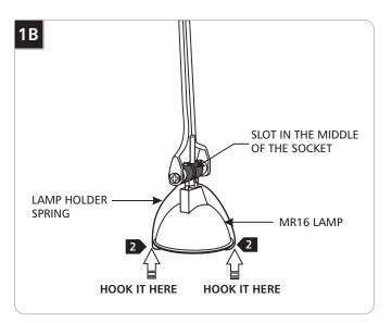
2 Hook one end of the lamp holder spring (provided with the package) onto front of the lamp. Wrap the spring over the slot in the middle of the socket and hook the other end onto front of the lamp.
