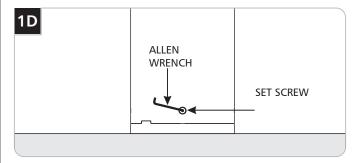
6 Carefully install the column assembly onto the base plate ans secure it in place by tightening all 4 set screws.
