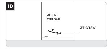
6 Carefully install the column assembly onto the base plate and secure it in place by tightening all 4 set screws.
