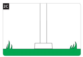
6 Stake the fixture to the desired location and properly bury the wire and wire nut connections.
