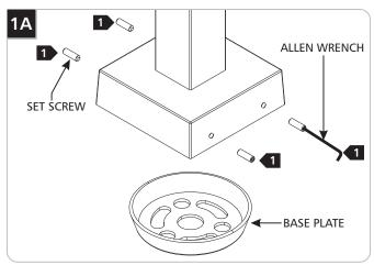
Loosen (**Do Not Remove**) the four set screws on fixture base with the provided Allen wrench and remove the base plate.
