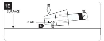
Tap the conical connector on a hard surface with the set screw facing down, so the plate inside drops into place.
