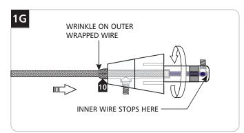
TO Keep pushing the coaxial cable into the connector while rotating the connector to ease feeding the inner wire into the tip of the connector. The outer wrapped wire will start wrinkling while being inserted another 1/2" into the connector.
