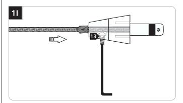
13 Firmly tighten the set screw on the conical connector.
