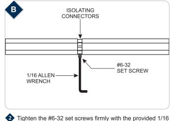
Tighten the #6-32 set screws firmly with the provided 1/16 Allen wrench. Do not overtighten the set screws or the threads may strip.
