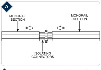
Push the two MonoRail sections completely onto the isolating connectors.
