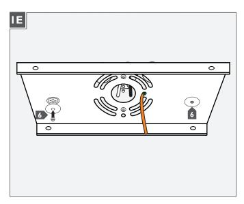
6 Secure the backplate to the anchors with screws and washers.
