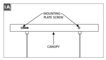
Separate the mounting plate from the canopy by removing all four mounting plate screws with a screw driver.
