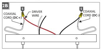
If shortening of the coaxial cords is necessary, take note of the wire connections and polarity from the coaxial cables to the driver and remove the wire nuts.
