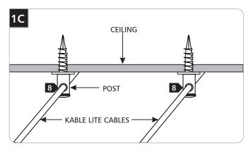
8 Feed the Kable Lite cables coming from one set of turnbuckles through the posts to the other set of turnbuckles.
