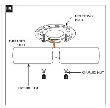
Remove the mounting plate from the fixture base by unscrewing the two knurled nuts from the two threaded studs.
