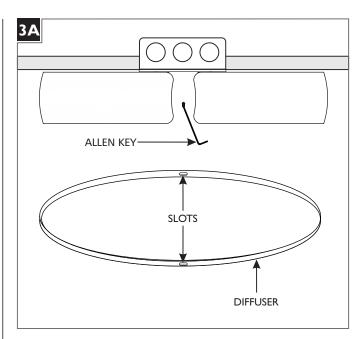
Install the diffuser by placing a diffuser slot onto the unloosened set screw, then align the other slot with the loosened set screw, and re-tighten the set screw using the provided Allen key.
