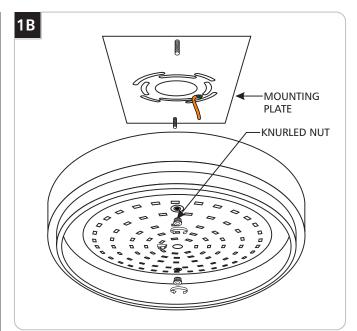
Remove the mounting plate from the assembly by unscrewing the two knurled nuts.
