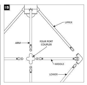
Install the remaining arms by inserting them into the four port couplers. Make sure arms are fully inserted.
