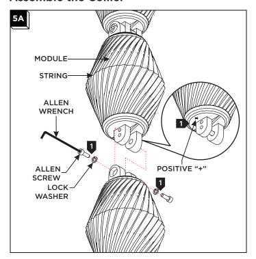
Connect strings together by using the washers and Allen screws making sure to match the polarity. Tighten the Allen screws until snug. Only connect up to 2' strings at a time (8 modules max).
