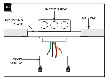
Secure the mounting plate to the junction box with the #8-32 screws.
