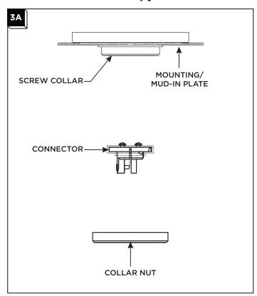
Remove the mounting/mud-in plate from the canopy by unscrewing the collar nut from the screw collar.
