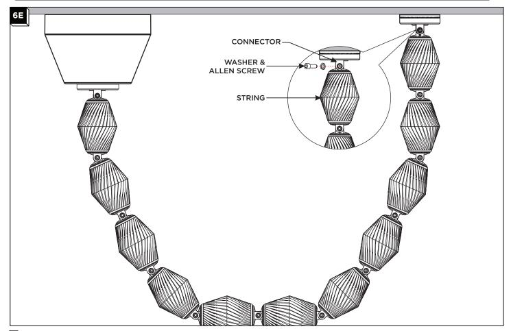
5 Connect the free end of a string to the standoff's connector using the washers and Allen screws.
