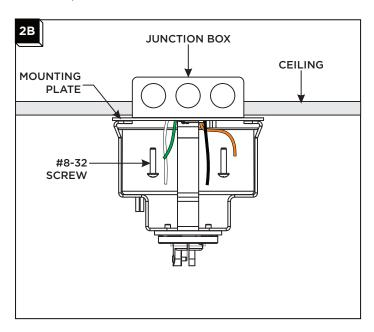
Secure the mounting plate to the junction box with the #8-32 screws.
