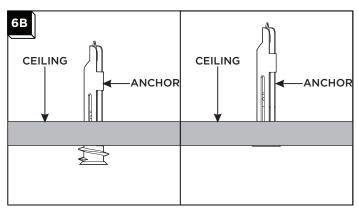
Install the anchor to the ceiling up to the threads. Screw it in the rest of the way.
