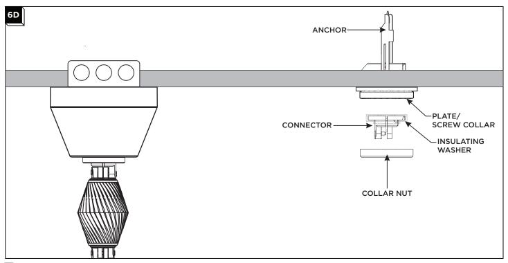
Insert the connector and insulator washer into the plate/screw collar and secure them together by screwing the collar nut onto plate/screw collar.
