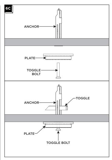
Place the plate/screw collar over the anchor head and secure it in place by screwing in the toggle bolt. Once the toggle bolt has been tightened, the toggle will secure the anchor inside the ceiling.
