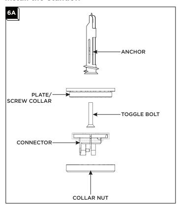
Disassemble stand-off assembly by unscrewing the collar nut and removing toggle bolt.
