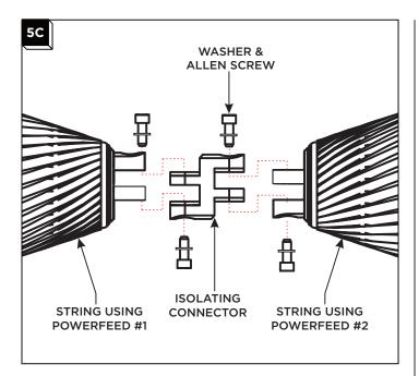
Use the isolating connector to connect two separately powered strings/fixtures using the washers and Allen screws. Tighten the Allen screws until snug.
