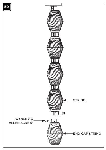
Install the end cap string to the end of a string using the washers and Allen screws making sure to match the polarity. Tighten the Allen screws until snug.
