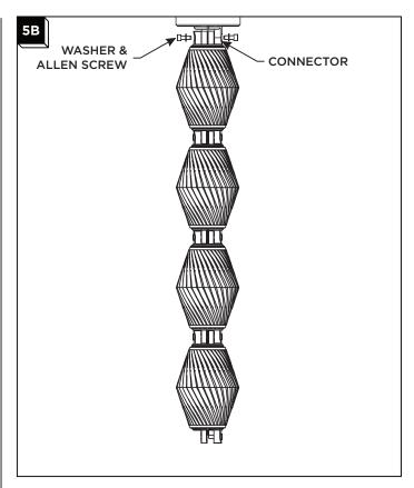
2 Install the increment to the connector using the washers and Allen screws making sure to match the polarity. Tighten the Allen screws until snug. Repeat as necessary. Do not attempt to hang the full length of string (more than 2' increments or 8 modules) at a time. Do not exceed a maximum of 20' of string per power feed point.
