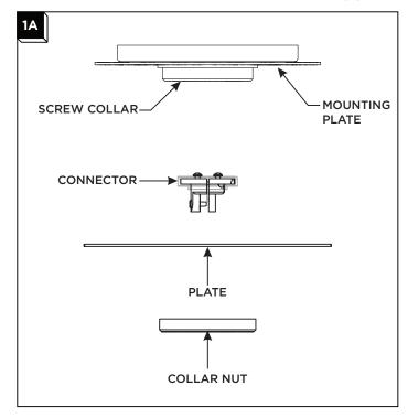
Remove the mounting plate from the canopy by unscrewing the collar nut from the screw collar.
