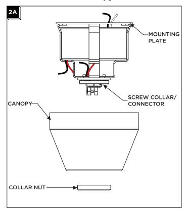
Remove the mounting plate from the canopy by unscrewing the collar nut from the screw collar/connector.
