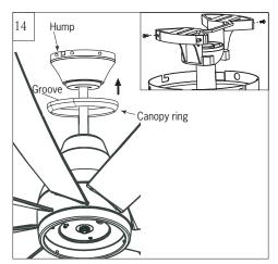
Partially loosen 2 of the set screws on mounting bracket corresponding to the slotted holes on the canopy upper ring. Remove the other 2 set screws. Save screws. Raise canopy to mounting bracket, aligning loosened screws in mounting bracket with slotted holes in canopy. Twist canopy clockwise to lock. Reinstall the screws just removed and then tighten all screw securely Install canopy ring onto canopy by aligning the grooves in canopy ring with the humps on canopy and snap it onto canopy.
