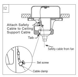
Connect the safety cable from fan to the Ceiling support cable.
