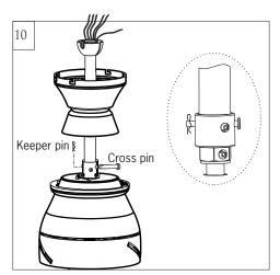
Slip downrod into motor yoke, aligning holes and install cross pin and keeper pin. Insert cross pin through yoke and downrod until point appears on the other side, and insert keeper pin on cross pin.
