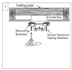
Use metal outlet box suitable for fan support and use only the screws provided with the outlet box (must support 35 lbs). Remove the two outlet box screws provided with the box, aligning the holes of the mounting bracket with the holes of the outlet box. Reinstall the 2 outlet box screws securely.
