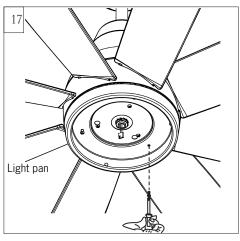
Loosen 2 and remove 1 preassembled screw from the light pan. Save screws for later use.
