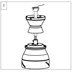
Thread lead wires and safety cable from motor assembly through downrod.
