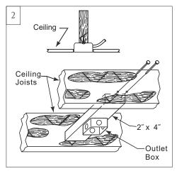
Before installing this fan makes sure the outlet box is properly installed to the house structure. Ensure the outlet box is securely fastened by at least two points to a structural ceiling member (a loose box will cause the fan to wobble). To reduce the risk of fire, electric shock, or personal injury, mount to outlet box or supporting system acceptable for fan support.
