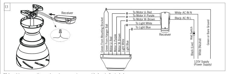
Make wiring connections using wire connectors provided as indicated above.
