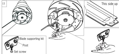
Preparing for blade installation, place a blade set screw into the blade supporting kit as shown in inset (**make sure the posts are downward**). Set screw provided. Insert a blade into the slot on flywheel (**hold the blade until at least one set screw is installed onto the flywheel**).
