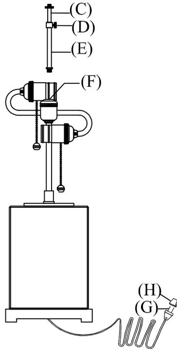
1. Thread rod (E) into top threaded opening of part (F).
