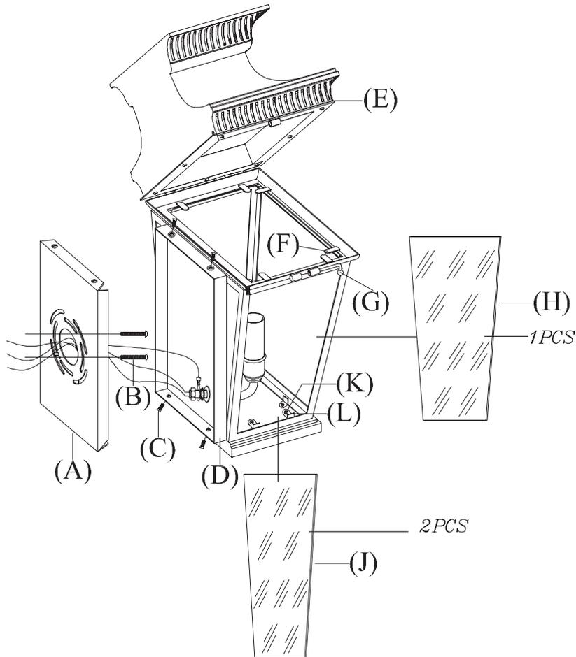
1. Remove mounting plate (A) from fixture base (D) by unscrewing base screws (C) in counter-clockwise direction. Attach mounting plate (A) to wall outlet box and secure with mounting screws (B).
