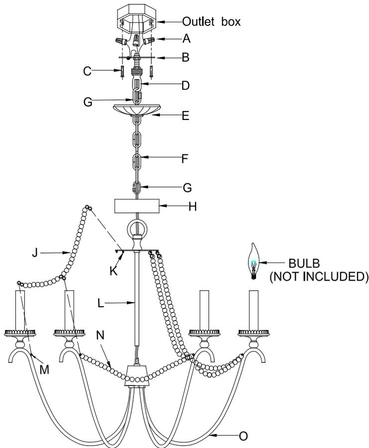
1. Thread the center tube (L) onto the nipple of fixture body (O). Slip the ring (H) to the disk with loop (K) on.
