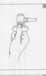
Turning off the water supply valves. This is usually found near the water meter. If you are replacing an existing faucet, remove the faucet from the sink and clean the sink surface thoroughly. You should clean all the dirts from valve outlets.
