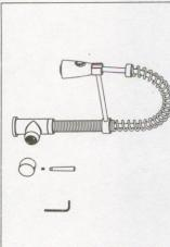
using a small flathead screwdriver, unscrew set screw using Allen Wrench and take off handle. Turn off water and relieve pressure! Detach handle button
