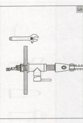
wrench until the faucet is firmly connected to the sink. If necessary, tighten screws using a adjustable
