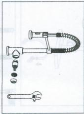
by hand. Unscrew Retaining Nut using adjustable wrench, take out cartridge assembly and inspect. Replace parts as necessary. Reassemble parts by reversing steps. Remove handles. Unscrew Dome Cap counter clockwise
