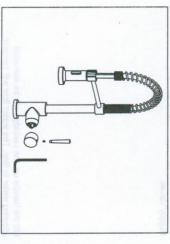
Turn off water and relieve pressure! Detach handle button using a ಇಲ್ಲಾ! ಗೆಲ್ಟ್ ead screwdriver, unscrew set screw using Allen Wrench and take off handle.
