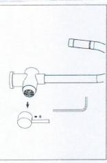
using Allen Wrench and take off handle. using a small flathead screwdriver, unscrew set screw Turn off water and relieve pressure! Detach handle button
