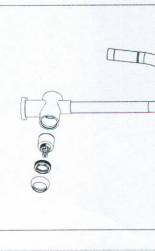
Remove handle. Unscrew Dome Cap counter clockwise by hand. Unscrew Retaining Nut using adjustable wrench take out cartridge assembly and inspect. Replace parts as necessary. Reassemble parts by reversing steps.
