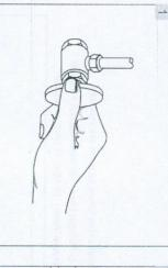
Shut off the water supply valves, remove the old faucet, rinse out the water lines and clean the sink mounting
