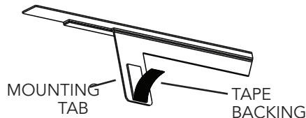
2. Peel backing from adhesive on the four (4) individual tabs.
