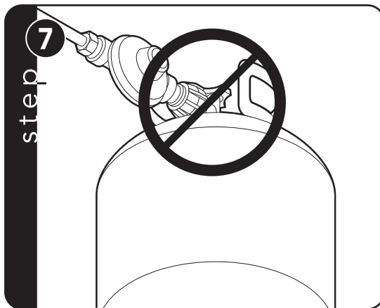
step 7 Do not attempt to repair the cylinder valve if it should become damaged. The cylinder must be replaced.
