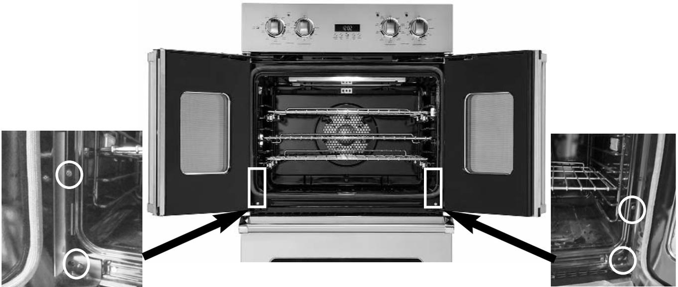
Using a 5/32" allen wrench, adjust screw on each door shown below moving the door that is too high downward and the door that is low upward. You want to adjust both in opposite directions, not just one door. Note that this moves the lower hinge assembly when adjusted.
