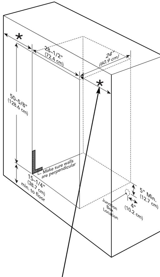
\*French Door Models (VDOF730/CVDOF730) must have a minimum of 18" (45.7 cm) clearance on both sides to allow for door swing.
